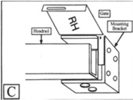
Push rail into brackets. Then press gate to close brackets.
