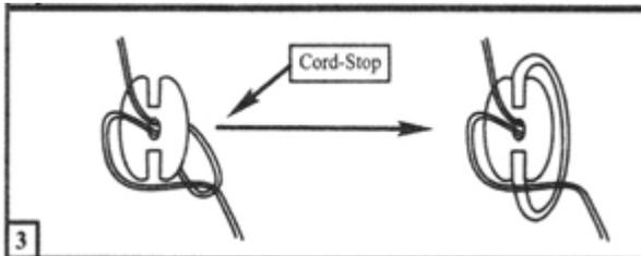
3. If cord-stops ARE NOT 1 to 2 inches below head rail, loosen (but do not untie) the knot surrounding the cord-stop.
