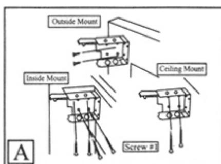
Brackets should be placed at the width of the blind's headrail, 6mm past each end. The bracket doesn't necessarily need to touch the inside face of the window frame.
