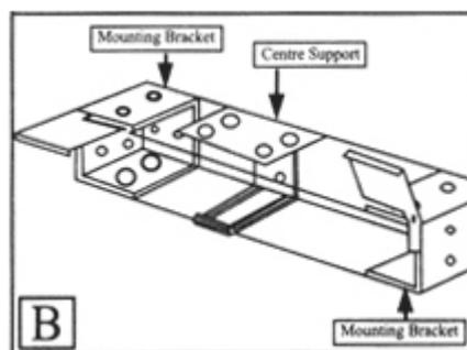
Align the top of the centre support bracket with the top of the mounting bracket before installation. Install with the bigger flap of the centre support bracket on the top side and clear of the slat ladder positions
