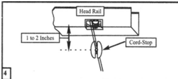
4. Push both the cord-stop and the loosened knot toward the head rail until the cord-stop is 1 to 2 inches below the head rail. Hold cord-stop in place and pull firmly on pull cord to re-tighten knot. Repeat steps 2, 3 & 4 for each cord-stop.
