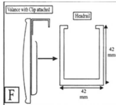
Hook valance clip with valance attached onto the top of the headrail.
