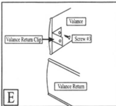
**For Outside Mount:** Screw one end of the valance return clip onto the valance using screw #3. Align the edge of the valance return with the valance. Screw the other end of the valance return clip onto the valance return.
